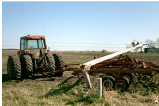
A primary line in northeast Kansas carrying 7,200 volts of electricity fell on this tractor when the driver came too close to the electrical pole.
